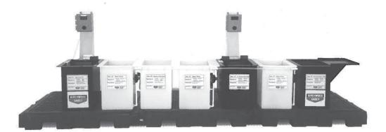
B&B Manufacturing has invested in a new Low Temperature Black Oxide line from Birchwood Casey. This system brings a previously outsourced process into B&B Manufacturing allowing us a cost-effective solution with a quicker turn around time. This particular system named TRU TEMP® provides a finish without Salt Bleed Out on all non-Stainless Steels and Cast Iron while remaining safe, operator friendly, RoHS compliant, and with no EPA problems.
